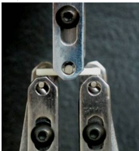
Figure 1- Bar-shaped specimen placed on the two jigs. Load was applied from the top by the blade for TPFS testing
